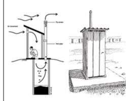
If the vent pipe is not covered by a gauze mesh or fly-proof netting, the facility should be classified as a pit latrine with slab not a VIP latrine. The inside of the VIP latrine is kept dark. If the door of the VIP superstructure is missing so that it is no longer dark inside the latrine, the facility should be classified as a pit latrine with slab, not a VIP latrine.
