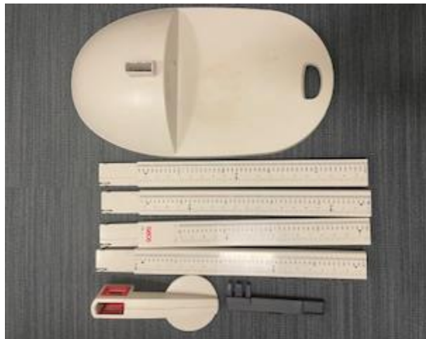
Figure 8 The foot piece, measuring rod (in four pieces), head piece, and wall stabilizer that make up the SECA 213 stadiometer
